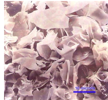
Perlite particles, after thermal expansion of the amorphous volcanic glass it is derived from
